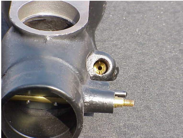
Reference the hole for the GAV assembly at the right (This carburetor has a brass GAV seat installed)
