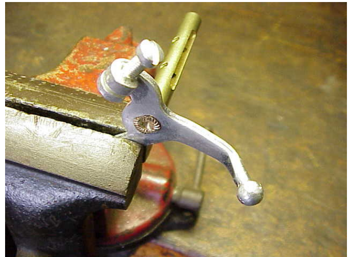
Arm curvature needs to be "carefully" bent more
