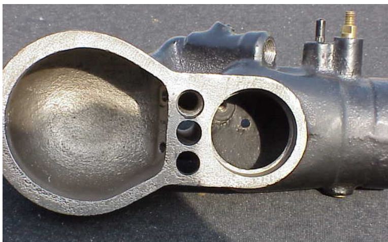
The secondary well is the hole at the top of the three vertical holes seen in the photo. The boss for the cap jet can be seen in the upper left of the venturi opening.
