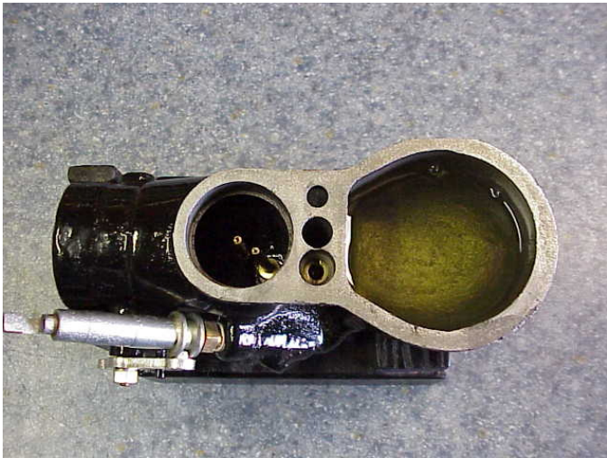
Testing for leaks at the GAV and main & cap jets
